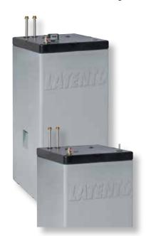
Unpressurized plastic storage tank as a buffer for recharging the boiler from different heat generating units. With integrated PUR insulation, gross volume 540 litres, with heat exchanger of long-wave stainless steel corrugated pipes for improved heat yield, external thread connector G  $1\frac{1}{4}$ .
